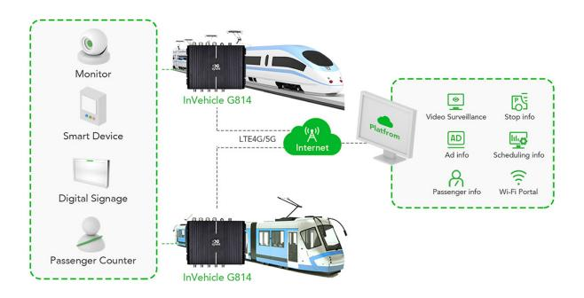
Devices on board, including monitors, smart terminals, digital signage, etc. are connected to the VG810 through extensive interfaces. Data from within the vehicles are collected and then sent out over high-speed 4G/5G networks. The VG814 can be easily integrated to 3rd party clouds, where data can be viewed and analyzed.
